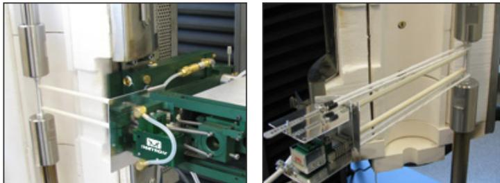
The extensometer and bracket mounts to the furnace or T-slot mounting arm and uses spring force to maintain contact with the specimen. The gauge length can be set prior to mounting; therefore, it can be mounted on specimens after they are heated, mitigating thermal expansion issues, and can be easily removed before fracture to prevent damage to the arms.
