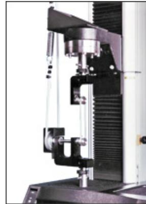
How to measure strain is important due to the nature of elastomers. Although many standards allow the use of crosshead displacement to measure strain, Instron recommends using an extensometer to measure the properties important to the customer.
