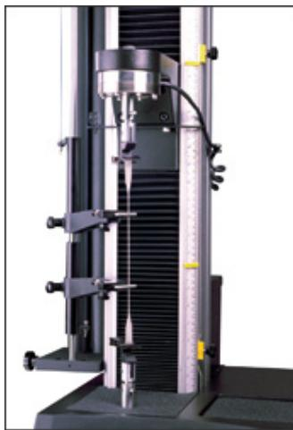
As previously mentioned, elastomers tend to thin as they elongate. This means if the crosshead displacement is used to measure strain then elongation is not only being measured at the gauge length but also outside the gauge length and within the jaw faces.
