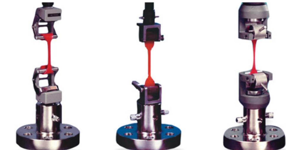
The self-tightening grips are ideal for meeting customers' elastomeric tensile testing requirements at ambient and non-ambient temperatures. These grips have a short effective length so that elongation in a chamber can be maximized.
