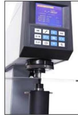
The supporting shoulder and the surface that the specimen sits on must be parallel to each other, and the anvil must present the test specimen perpendicular to the indenter. Both the supporting surface and the shoulder must be free of nicks, scratches and dirt, and be of sufficient design to properly support the material under test. You should examine anvils regularly, typically prior to each use, and replace them when necessary.
