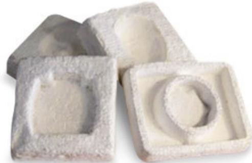
Until recently, there has been little alternative to Styrofoam, in particular for protecting heavy items such as appliances and furniture from shipment damage. Enter Mycobond™, a new biodegradable biocomposite material developed by Evocative Design LLC of the aptly named Green Island, NY.
