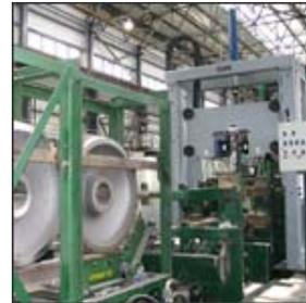
ASTM standard E103: Standard Test Method for Rapid Indentation Hardness Testing of Metallic Materials details this test type. The systems can be integrated to production automation lines or can stand-alone. They are customizable to meet many application requirements.
