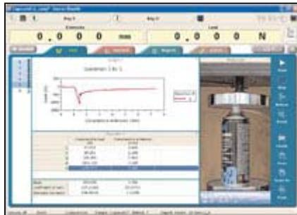
The video capture module in Bluehill 2 simultaneously records the entire test from start to finish along with the test data points. The video capture feature of the test, with an on-demand replay, allows you to easily review the test down to the finest detail and time frame. After testing, a scanning cursor allows you to select particular points of interest while viewing the associated test video frame. Additionally, the video can be stored and sent electronically.
