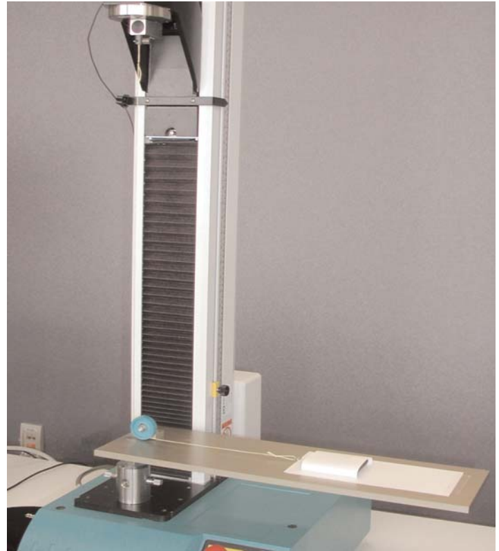
▲ Figure 1: Test configuration for coefficient of friction test between two sheets of copy paper.
