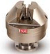
Side-entry wedge grips for use with ElectroPuls systems have been designed to combine low mass with excellent gripping performance for a range of static and fatigue tests. Available in both manually-operated and pneumatically-operated wedge grips, the range of jaw faces allows for testing of various specimen types and thicknesses. It's important to note that Pneumatically-operated grips require a suitable air kit and air supply.
