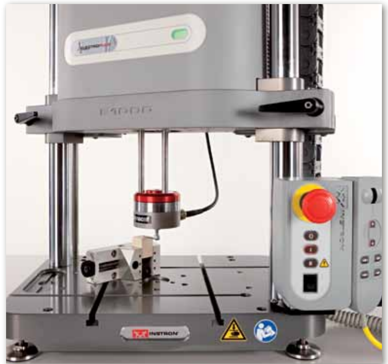
Fatigue tests of fixation devices for phalangeal, metacarpal, and carpal bones tested on ElectroPuls™.
