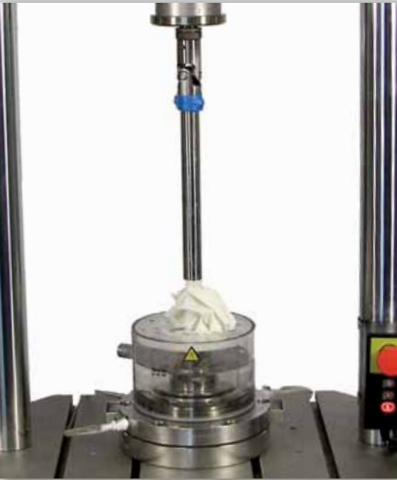
Combined axial and torsional loadings can be applied to intervertebral disc replacements according to ASTM F2346.
